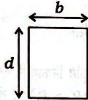
Moment of inertia of rectangular section shown in the above Fig. about its base is
