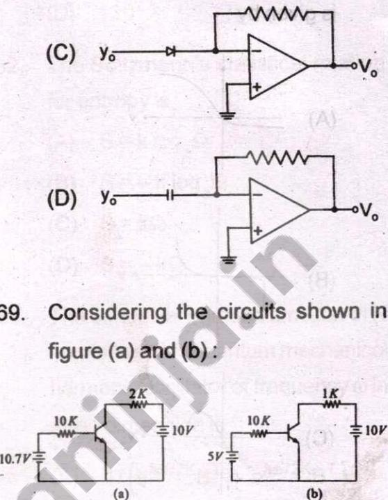
If the transistor in figures (a) and (b) have current gain ( $\beta_{dc}$ ) of 100 and 10 respectively, then they operate in the :
