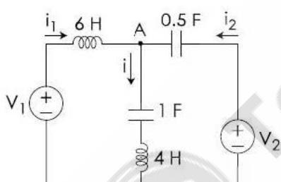
In the circuit  $V_1=6 \cos\omega t$  and  $V_2=\cos(\omega t + 60^\circ)$ . Find  $V_A$ , if  $\omega=2$  rad/sec.
