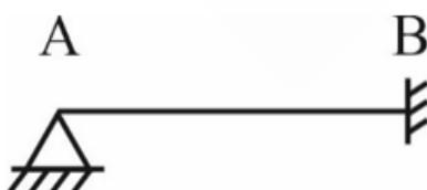
The beam is subjected to a moment  $\mu$  at the hinged end. Due to moment  $\mu$ , the end A rotates through angle  $\theta$  while rotation at end B is zero.  $\mu'$  represents induced moment at end B. Which of the following is correct?
