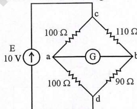
The internal resistance of the galvanometer is 1 ohm. Using Thevenin's theorem, determine the galvanometer current.
