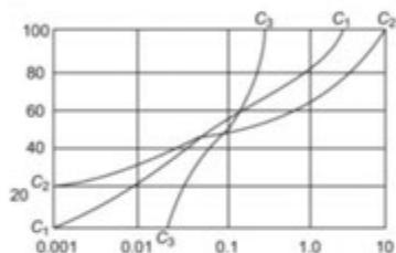
The above given figure is a Grain size distribution curve of different type of soils. What type of soil does the curve  $C_1C_1$  represent?
