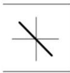
The above Lissajous pattern is observed in CRO. What is the phase difference between the applied signals?
