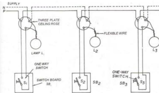
Identify the method of representation for wiring diagram as depicted above.
