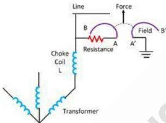
Identify the type of lightning arrester from the above figure.
