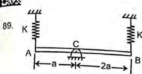
89. A rigid uniform rod AB of mass m and length  $3a$  is hinged at C as shown in the figure. It is supported by springs of spring constant K at the ends. Natural frequency of the system is given by
