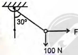
A rigid ball of weight 100 N suspended with the help of a string. The ball is pulled by a horizontal force  $F$  such that the string makes an angle of  $30^\circ$  with the vertical. The magnitude of force  $F$  is
