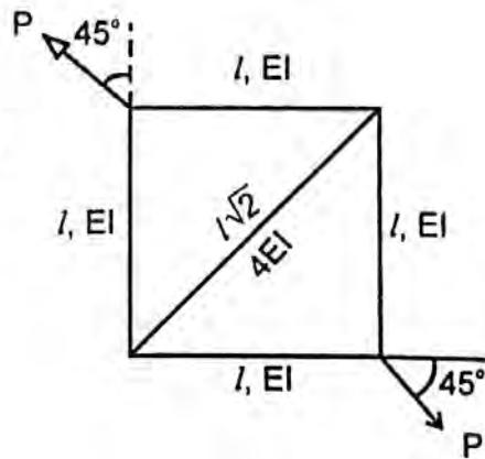
A truss shown in figure has 4 members of length 'l' and flexural rigidity 'EI' and one member of length,  $l\sqrt{2}$  and flexural rigidity,  $4EI$ . The truss is loaded by a pair of forces of magnitude P as shown in figure. The smallest value of P to initiate buckling in some member is
