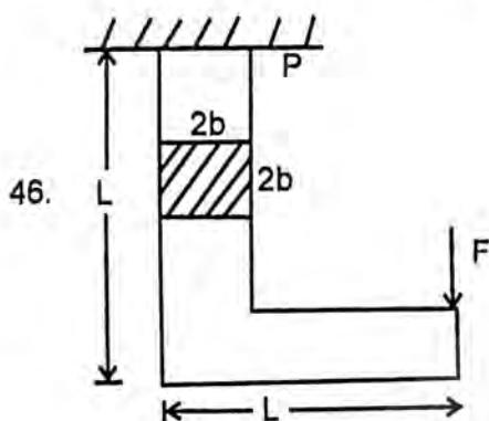
46. For the component loaded with a force  $F$  as shown in the figure, the axial stress at the corner point P is
