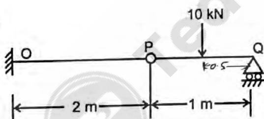
A cantilever beam OP is connected to another beam PQ with a pin joint as shown in the figure. A load of 10 kN is applied at the mid point of PQ. Magnitude of bending moment, in kNm at fixed end 'O' is
