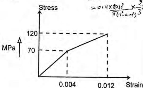
Stress strain behaviour of a material is shown in the figure. Its resilience and toughness, in  $\text{Nm/m}^3$ , are respectively
