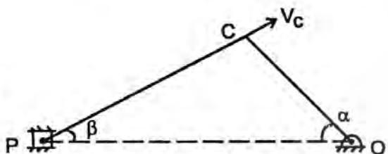
The cross head velocity in the slider crank mechanism for the position shown in the figure is
