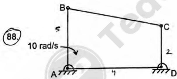
In a four bar planar mechanism, ABCD, as shown in the figure,  $AB = 5$  cm,  $AD = 4$  cm and  $DC = 2$  cm. In the given configuration, both AB and DC are perpendicular to AD. Bar AB rotates with angular speed of  $10$  rad/s. At instant, angular speed of the bar CD in rad/s is
