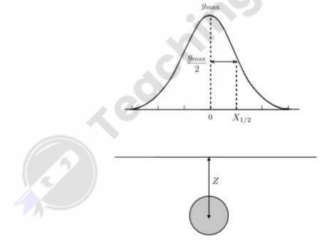
Q.73 Two survey vessels with shipborne gravimeters are cruising towards each other at a speed of 6 knots each along an east-west course. The difference in gravity readings of the two gravimeters is 63.5 mGal at the point at which the survey vessels cross each other. The latitude along which the survey vessels are cruising is \_\_\_\_\_\_°N.
